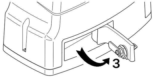
Turn the lock cover (ref. **1**), insert the key included in the lock and turn clockwise by 90° (ref. **2**), then pull the key first and then the lever to open the door (ref. **3**) completely.
